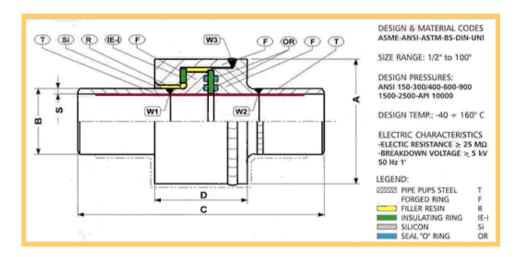
Monolithic (one piece) Insulation/Isolation Joints
